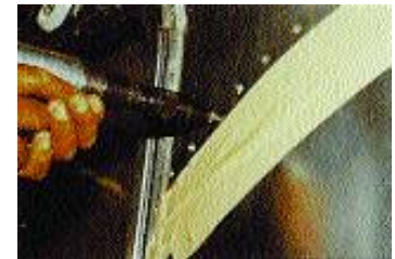
2. PROPER SIZED SHAPER TOOL, INSTALLED IN A STANDARD 1/4" DRILL, SHAVES RIVET HEAD.
